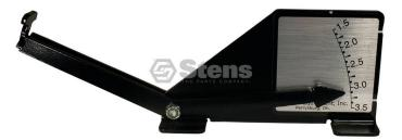
Leveling Gauge Universal Used to accurately level and measure mower decks on all riding and walk behind mowers Used to accurately level and measure mower decks on all riding and walk behind mowers Measure tip to tip cutting edge (side to side and front to back)- Measure one side cutting edge. Check height on gauge- Measure other side cutting edge. Check height on gauge.- Deck is level if heights are the same. If not, deck adjustments will need to be made.USE GLOVES TO AVOID INJURY
