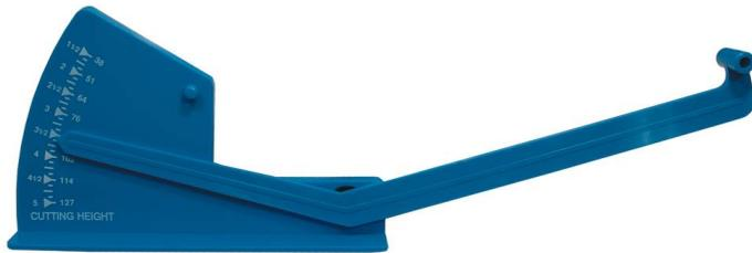
Leveling Gauge Plastic Plastic Used to accurately level and measure mower decks on all riding and walk behind mowers Mower blade cutting height gauge range is 1 1/2" to 5" Measure tip to tip cutting edge (side to side and front to back)- Measure one side cutting edge. Check height on gauge.- Measure other side cutting edge. Check height on gauge.- Deck is level if heights are the same. If not, deck adjustments will need to be made. USE GLOVES TO AVOID INJURY
